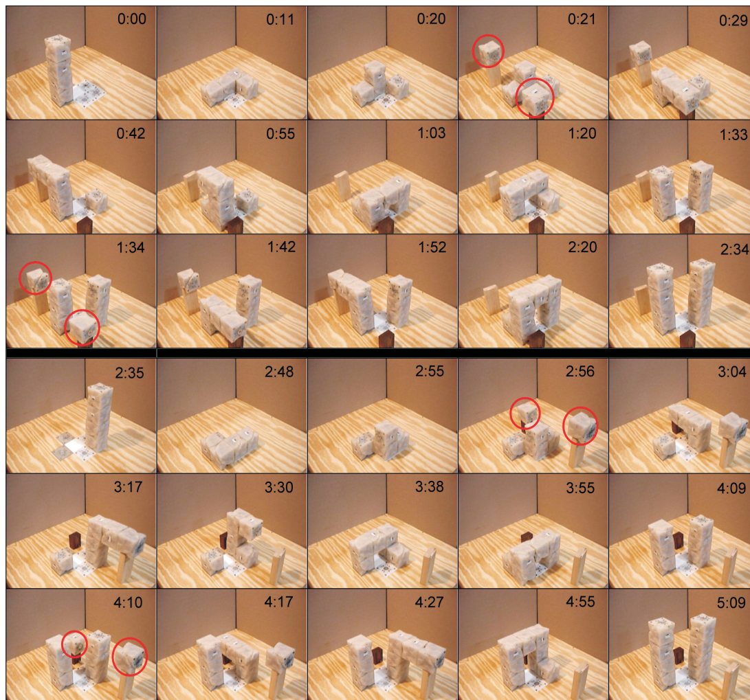
Figure 5.3: Reproducing robots developed at Cornell University by Zykov, Mytilinaios, Adams, and Lipson (reproduced with permission) [170]. Each cube is a robot. The 4-module conglomerate robot in the top-left frame moves through a variety of configurations, collecting other cubic robots from its environment (encircled in red), in order to create a copy of itself, visible in the bottom-right frame.
